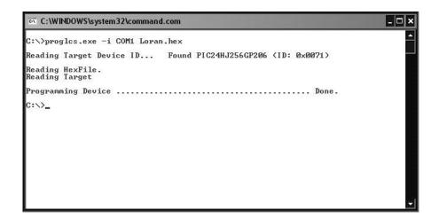
4.1.5 After the update, turn the LCS-300 power off for a second then back on before using it. You may verify the software version by typing a 'v' then pressing 'enter'. The software version will be displayed on the terminal.
