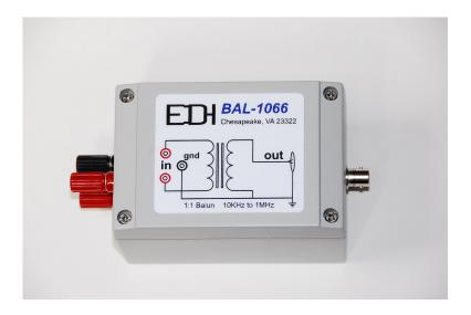
The BAL-1066 is a high power balanced to unbalanced line transformer designed for operation down to 10 Khz. It also provides galvanic isolation between input and output. This balun is used to connect depth sounders to the DSTS-4A, DSTS-5A, and DSTS-5A/2C Chirp depth sounder test sets.
